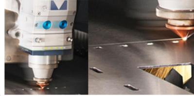
• Enhanced Gas Control System Allows the use of higher presssures to facilitate the cutting of thicker stainless steel
