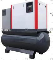
Assist air cutting compressor - Max 1.8 MPa (18 Bars) pressure for assistant cutting gas for thin material and any thickness for Aluminium material, copper and brass. The compressor is 4 in one package, i.e. compressor, air Cooling (drying) system, high pressure accumulation tank and oil filter/water filter system.
